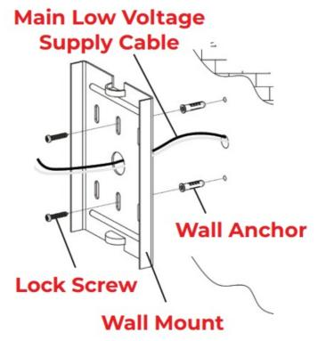
Place the wall mount at the desired location and mark two points on the wall surface for the wall anchors.
