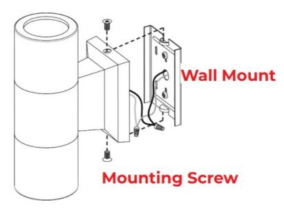
Carefully tuck all the wires into the wall mount. Attach the back of the luminaire over the wall mount. Secure it by threading the mounting screws onto the top and bottom of the luminaire body.
