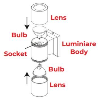
Insert the bulbs (sold separately) with the correct wattage and type marked on the luminaire label.
