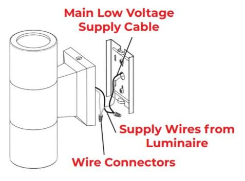
Using two wire connectors (sold separately) connect the supply wires from the fixture to the main low voltage supply cable leads.
