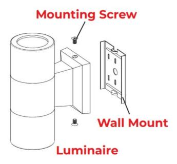
Remove the mounting screws off the top and bottom of the luminaire and remove the luminaire from the wall mount.
